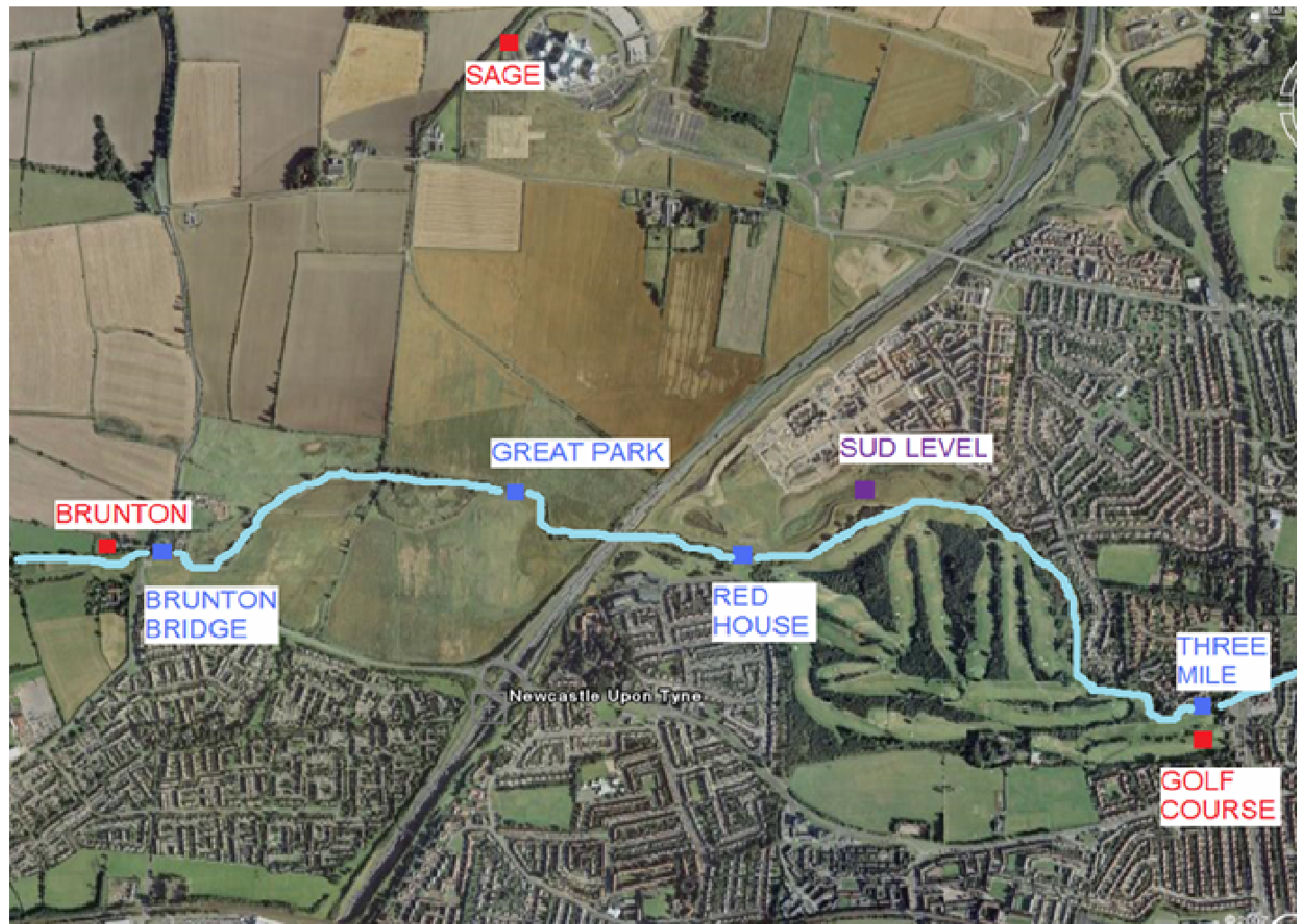
Figure 2.4:- An areal photo displaying the location of Newcastle University Hydrometry in the upper Ouseburn catchment where red squares are raingauges, blue squares are gauging stations and purple squares are SUD water level loggers (Taken from Google Earth).
