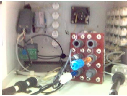
Aqualab analyser for TDP analysis, Nitrate, ammonium, turbidity, EC, pH, DO & temp
