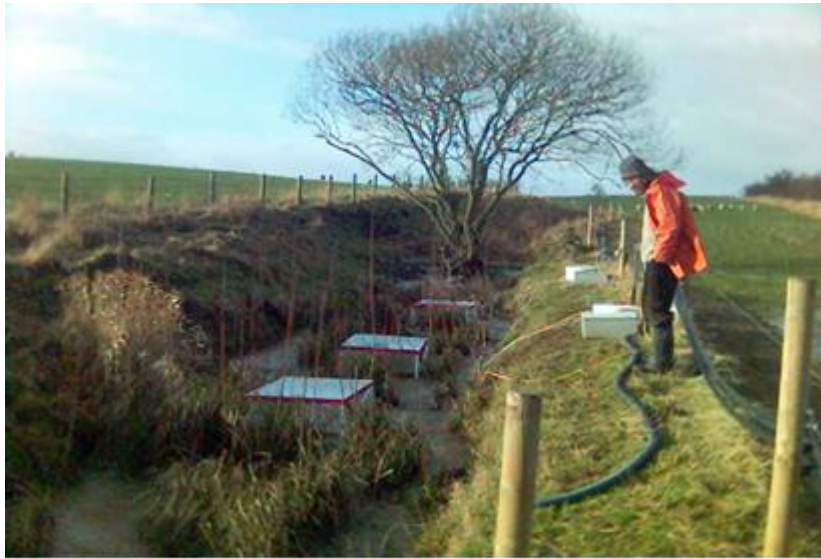
Fig. 2. 8 Sedge wetland instrumented with rice chambers for investigation of gaseous emissions by Edinburgh University.
