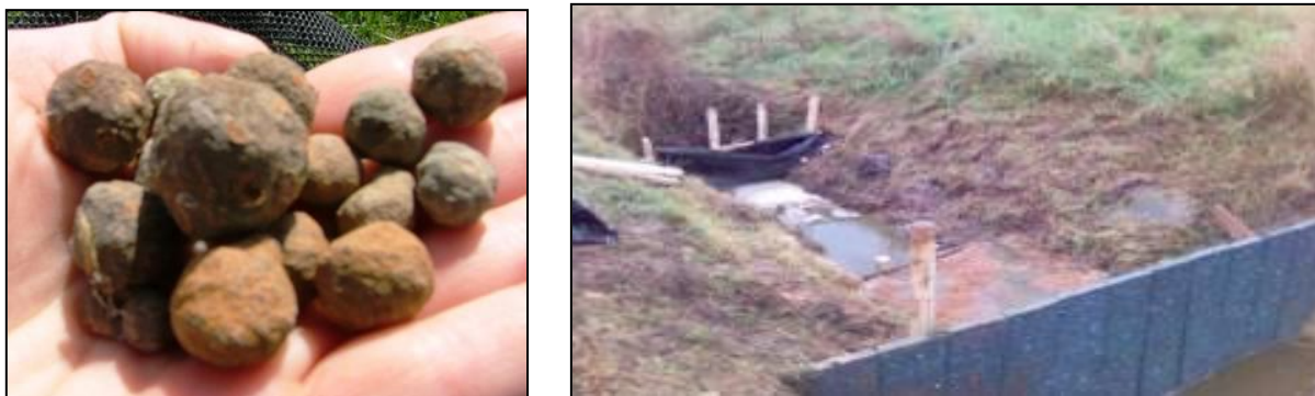
Figure 3.13. Ochre pellets and the phosphorus trap
