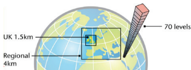
Figure 2: Model configuration used for operational weather forecasting at the UK Met Office
