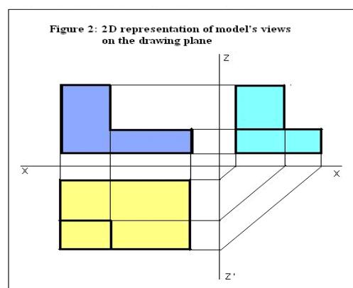
intuitive ability to identify the best viewing direction for good representation and thus the easier solution of spatial problems as in the above 3D mode\* shown in figure 1 in simple axonometric projection. Thus, modelling and model manipulation are key skills worth mastering in order to be able to
