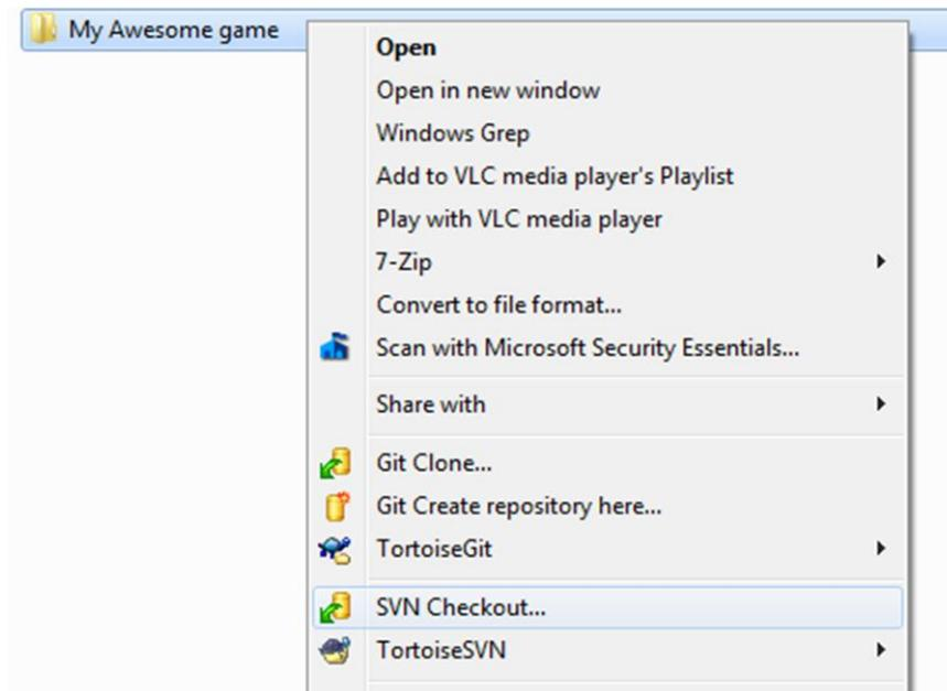
*Step 1: Decide where to checkout the SVN to. With TortoiseSVN installed, click the destination folder, and select the new 'SVN Checkout' option*
