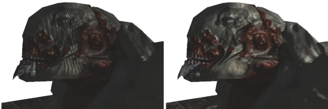
Left: An example of 'surface acne' and Right: Vertex offsetting reduces the acne effect
