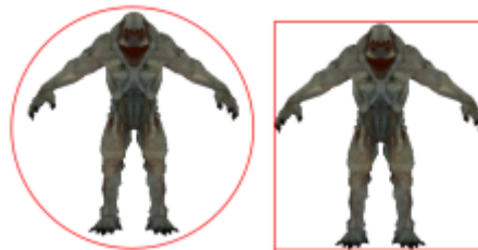
An example game character and two example bounding volumes, a sphere and a box
