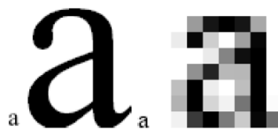
Example of Vector graphics being smoothly rescaled. Left: Vector Graphic Right: Bitmap
