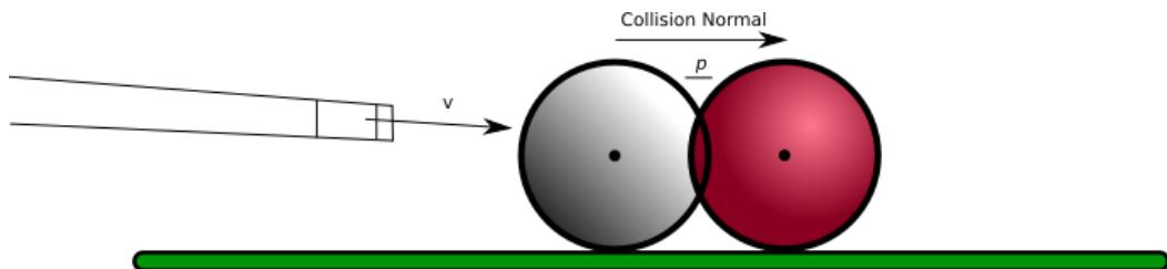
We can then 'solve' the collision by separating them out along the contact normal:
