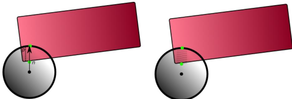
We can state that the temporary spring has a resting length of *zero*, and that it is being extended along the collision normal  $n$  by the penetration distance  $p$ . From this, we can apply a force proportional to the penetration distance, at the collision point on each object, in the direction of the collision normal
