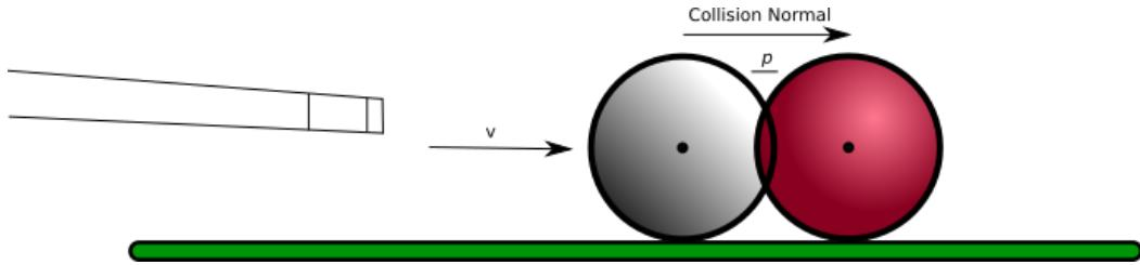
As the projection method doesn't take into account the relative velocities, or masses, between the objects, its not particularly suitable on its own. Consider if instead the cue ball hit a *planet* - the projection method would just move both the planet and the ball along the collision normal by the same amount, and the physical accuracy of the simulation would be lost.
