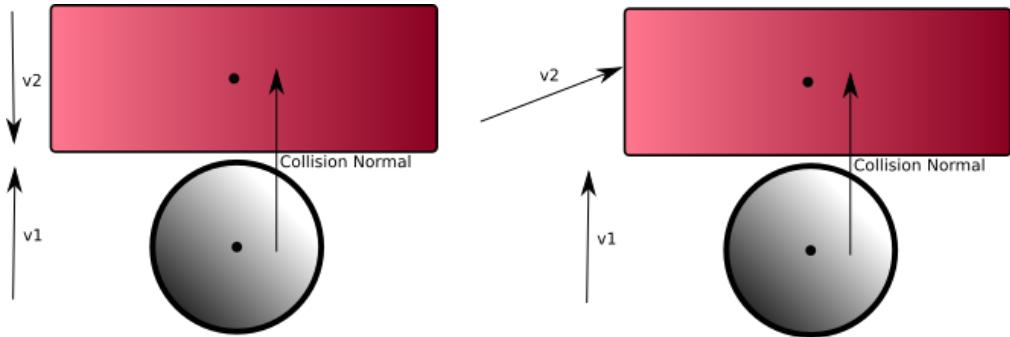
In both cases the relative velocity between the objects is the same, but in the right case the objects are only narrowly colliding in the direction they are traveling in, while on the left the collision normal matches up to the direction being traveled in, and so should result in more energy being transferred.
