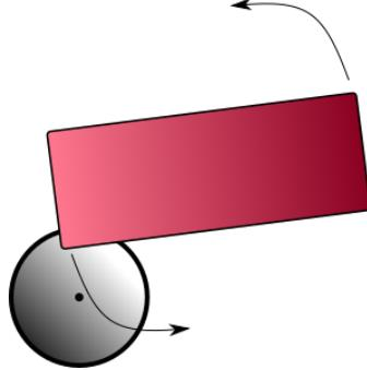
Imagine that neither the sphere or the box are moving in space (their *linear* velocity is zero), but that the red box is spinning around. At some point the box will collide with the sphere, generating a contact point on the edge of the box. Clearly, the sphere must be knocked downwards by the spinning box, but as so far we've only been considering linear velocity in our impulse  $\mathbf{J}$  will in this case have a magnitude of zero, and nothing will happen.
