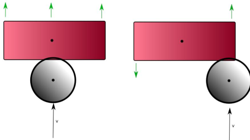
In the left example, the sphere is hitting the cuboid straight on, and it seems intuitive enough that the cuboid will be pushed away. In the right example, the sphere is hitting the corner of the cuboid, and the 'correct' thing that would occur would be that while neither the sphere or the cuboid had any angular motion at the point of collision, that the cuboid should 'twist' under the impact - these expected results are indicated using green arrows in the example.
