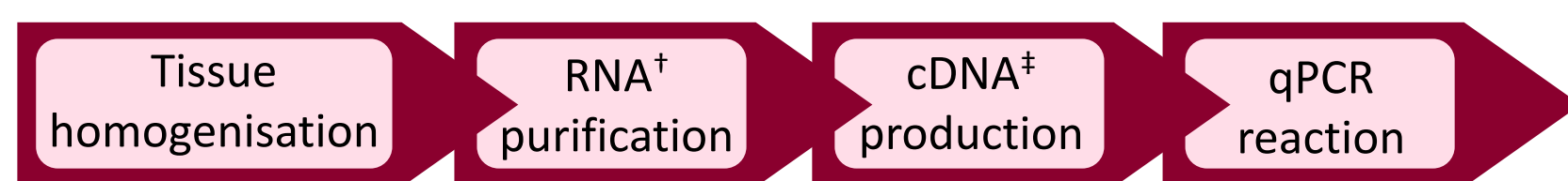
Figure 3: Preparation process for qPCR. Solid tissue was shredded to enable RNA extraction. † RNA is a macromolecule which aids in synthesising proteins. ‡ cDNA is a genetic material synthesised from RNAs, which is used to carry out qPCR.
