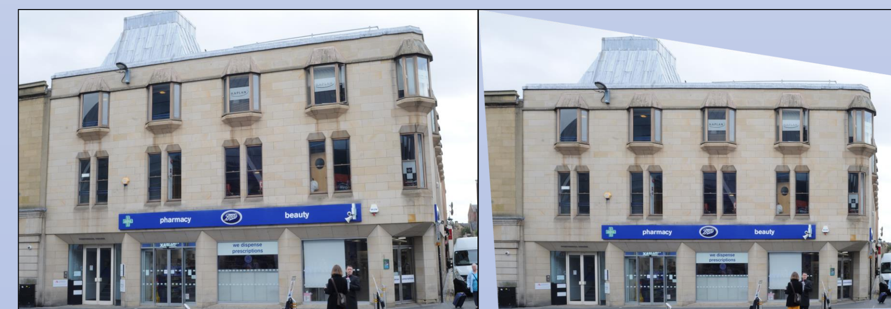
Figure 3: Example results of the correction performed on the facade photographs. Left - pre-correction. Right - post-correction.
