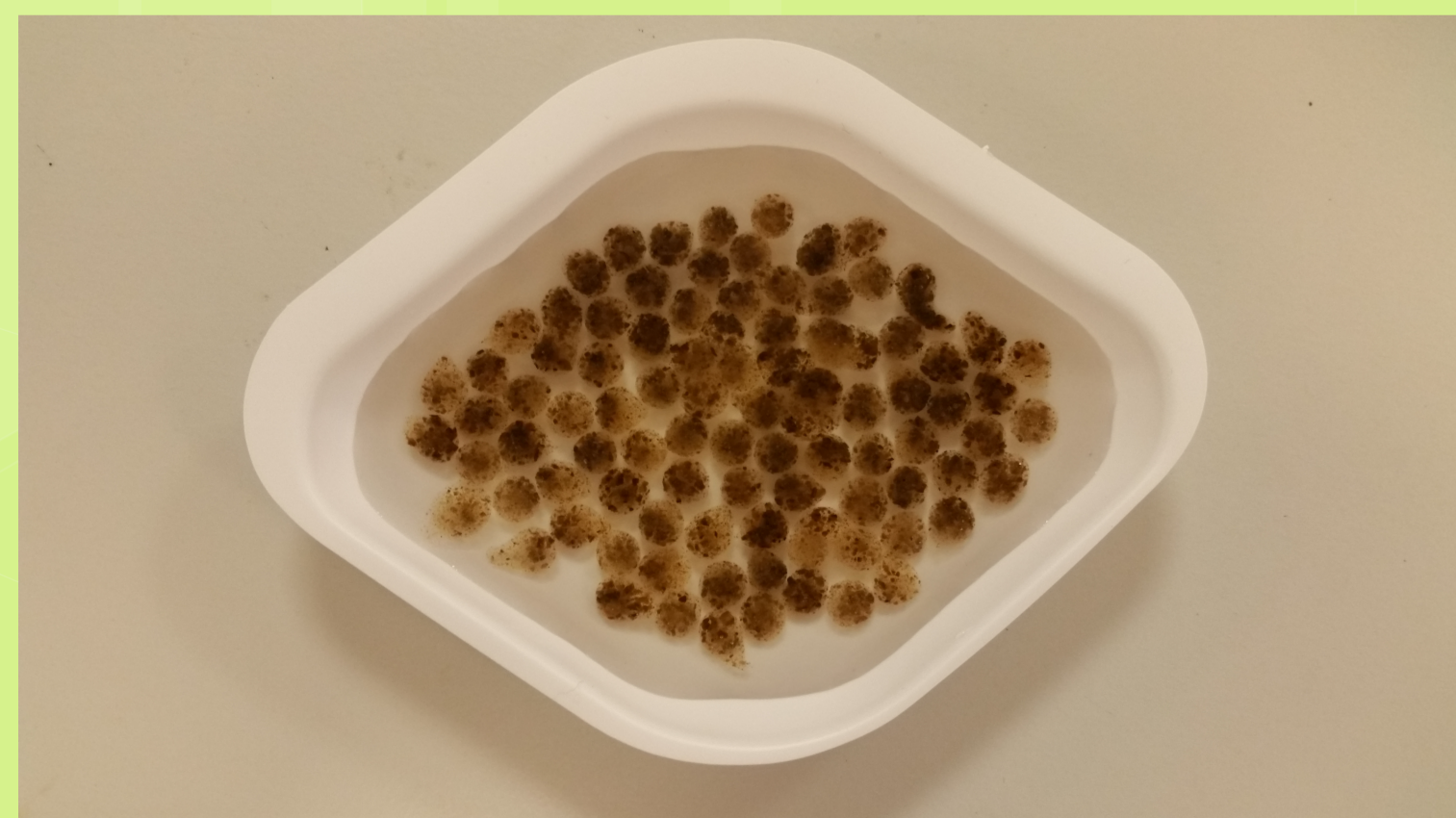
Picture 1: Beads were made in a ratio of 2:3 alginate and Calcium Chloride.
