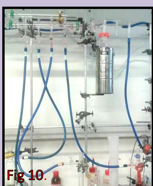
Fig.10 A Schlenk line provides an inert atmosphere.
