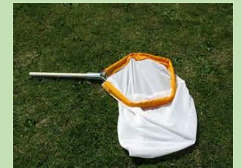
Fig 3: The type of sweep net used to collect the airborne and vegetation invertebrates (NHBS supplies)
