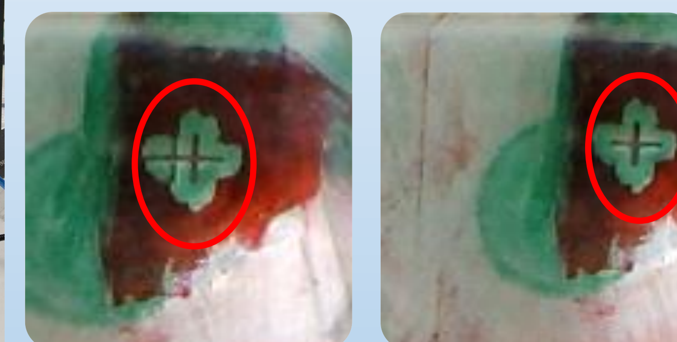
Figure 4. Illustrates two alignment marks prior and after alignment
