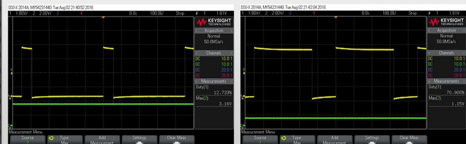
Figure 2: When the input voltage is high (3.16V; green trace), the duty cycle of the PWM output is low (12.7%; yellow trace)
