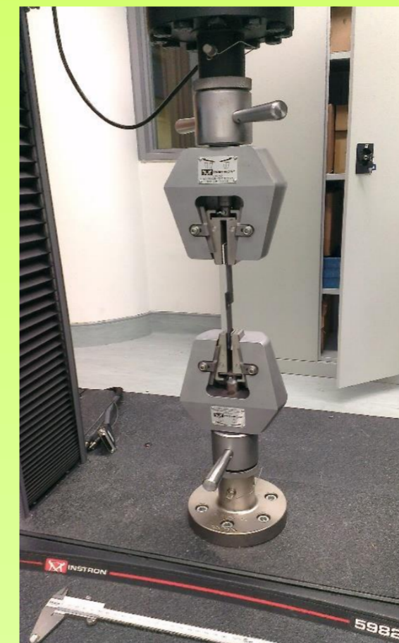
Fig. 5 Specimen mounted on the Instron 5982 universal testing machine.
