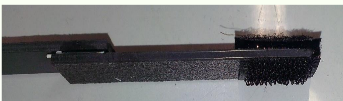
Fig.3 Velcro glued to grip area adding more friction to grip.
