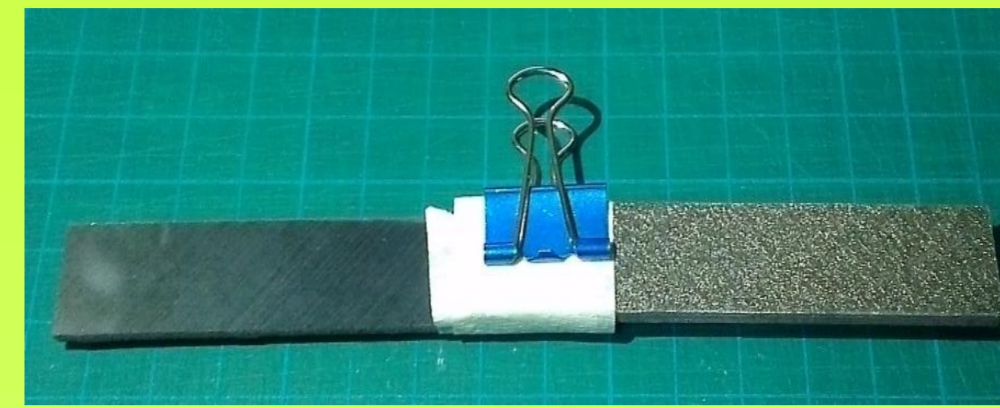
Fig. 4 Specimen wrapped in tape and aluminum clip to hold in place.
