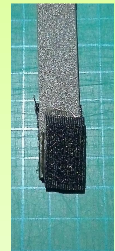
Fig. 7 The Velcro material glued to the composite starts to peel off.
