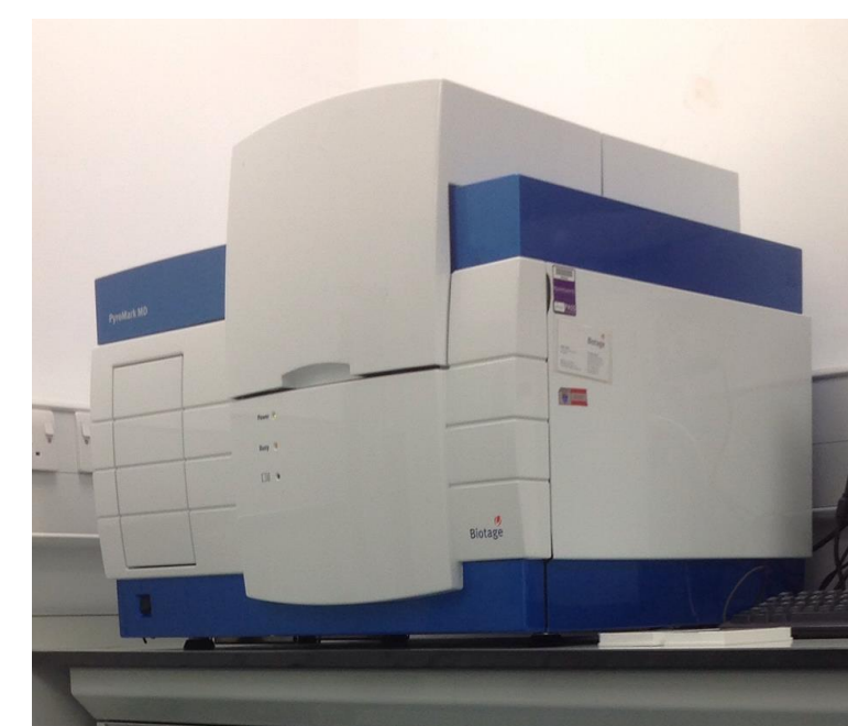
Figure 3: The pyrosequencer housed in the Centre for Aging and Vitality. Pyrosequencing is a form of DNA sequencing which relies on a chemical reaction producing light from with the addition of each correct complementary base pair to the template sequence. This occurs by a series of reactions beginning with the release of PPI from the DNA strand, which is converted to ATP and then used as a coenzyme to luciferase to produce light from luciferin.
