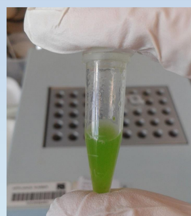
Figure 2. 'green soup solution' in an eppendorf tube heated to 60°C for 25 minutes
