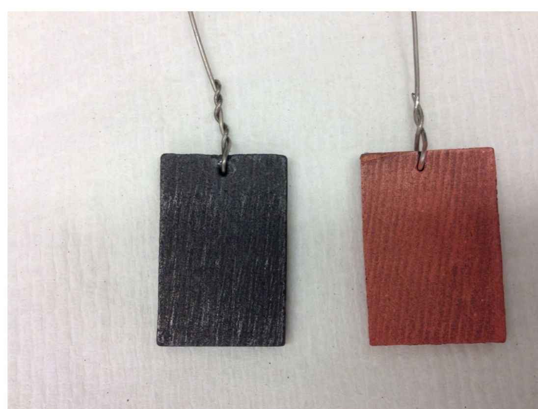
Working electrode at t=0 (left) and t=48\text{h} (right)
