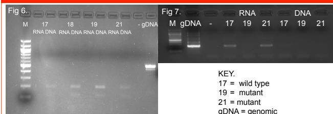
Having optimised and identified primers, RNA was reverse transcribed to make cDNA and then PCR amplified to assess RNF220. See RT-PCR gel Fig 6. To test for inclusion of introns, I used primers from exon 6 to exon 7 in RT-PCR on fetal kidney RNA from mutant (17 18 wt, 19,21 mut) and wild type. There is no evidence of DNA contamination in RNA samples as seen by the empty lanes. There are two different forms of RNF220 expressed in both wt and mut (this is OK with ensemble). There is also no evidence of intron inclusion because there are no bands of the same size as genomic DNA. Fig 7. To further test for inclusion of introns, I used primers located within intron 2 (primer set 7) in RT-PCR on fetal kidney RNA from mutant and wild type. Empty lanes means there is no evidence of DNA contamination in RNA samples but there is some evidence of expression of the intron sequence in samples 17 and 21. However this does not vary with genotype. I have discovered RNF220 does have retained introns but this does not seem to be 100% associated with the mutations. Therefore it is unlikely to be involved in CKD predisposition. But more samples may reveal some association.
