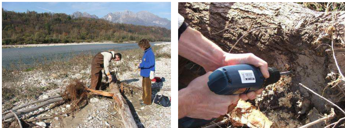
Figure 15 – Installation of radiotransmitters into the selected logs.
