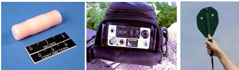
Figure 12 – The radiotransmitters, receiver and antenna used in this research.
