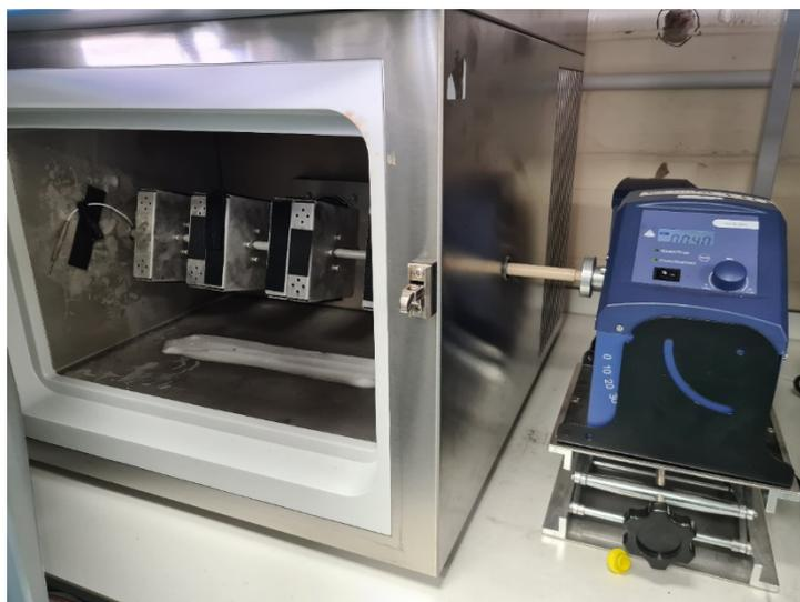
**Figure S4:** Ampoules were loaded onto metal plates which were fitted to the rotator axel. The axel passed through factory adapted ports in the sides of the incubators, in this fashion the electric rotator could safely be sited outside of the extremes of temperature. Temperatures were monitored with probes passed through the same ports.
