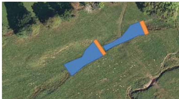
Diagram showing the indicative storage potential of the two bunds. Taken from the proposals document 'multiple track bund features'
