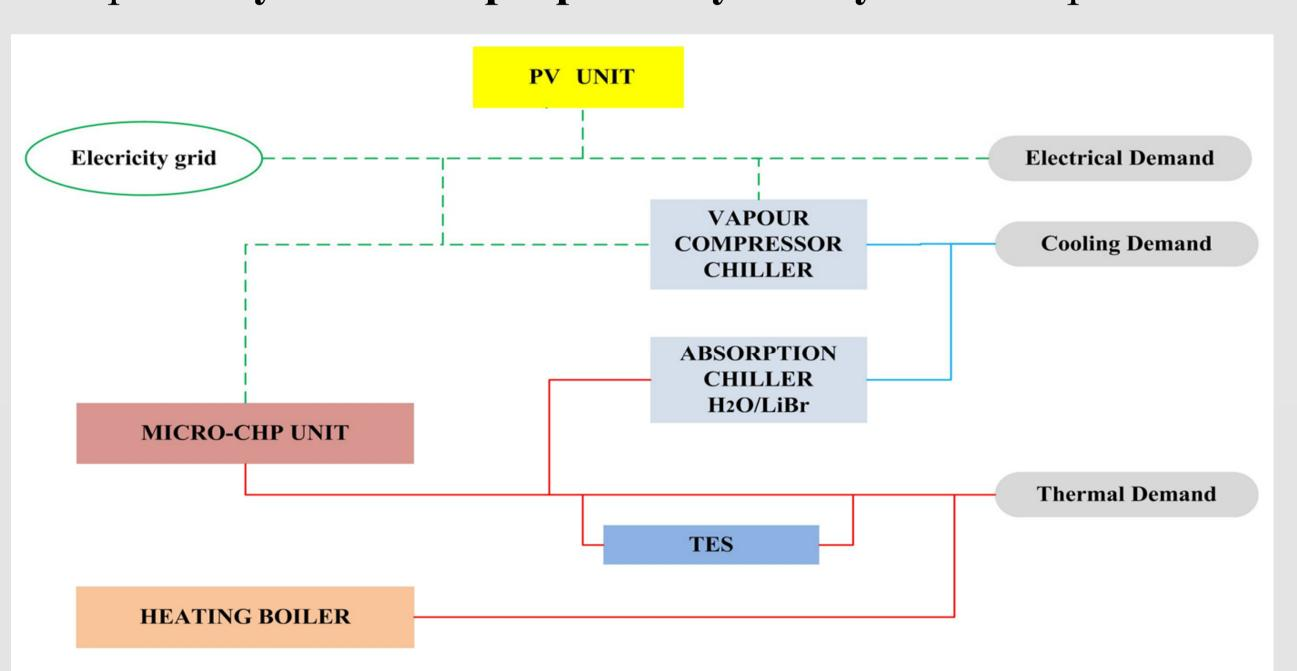
Figure 1 – Hybrid system layout
