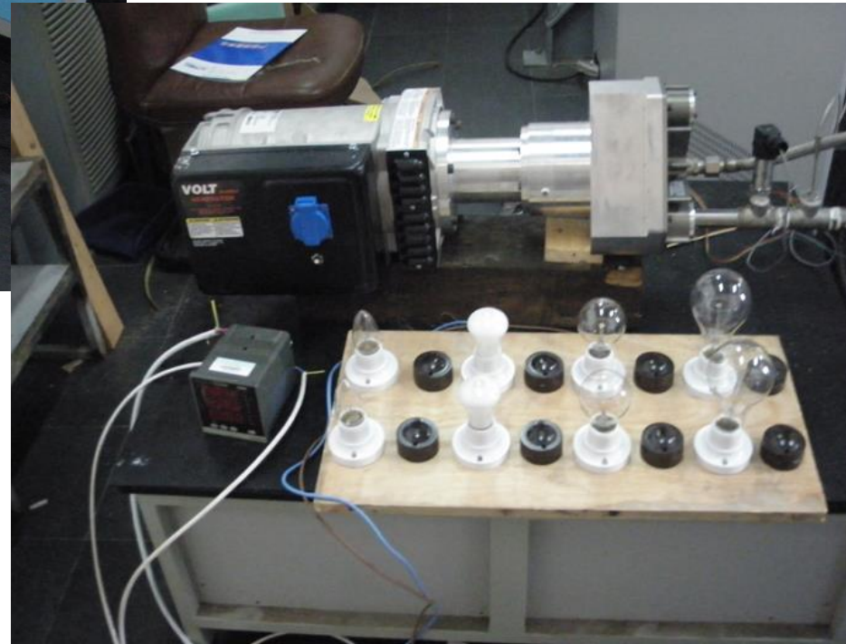
Light bulbs as load bank
